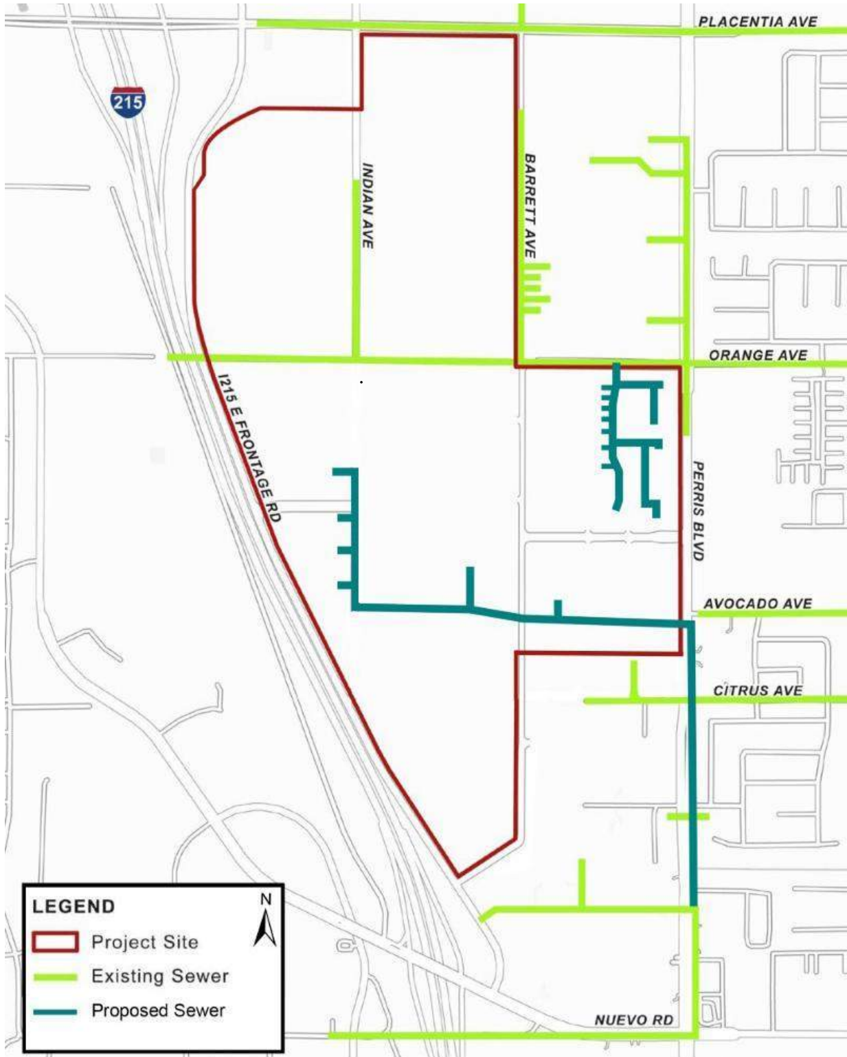
Figure 3.0-11, Existing and Proposed Sewer Infrastructure
