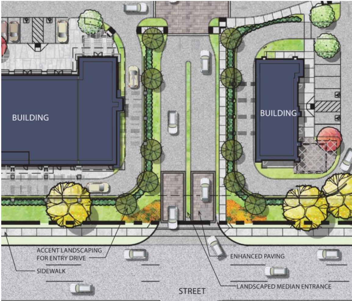
Figure 5.0-15, Enhanced Driveway Features
