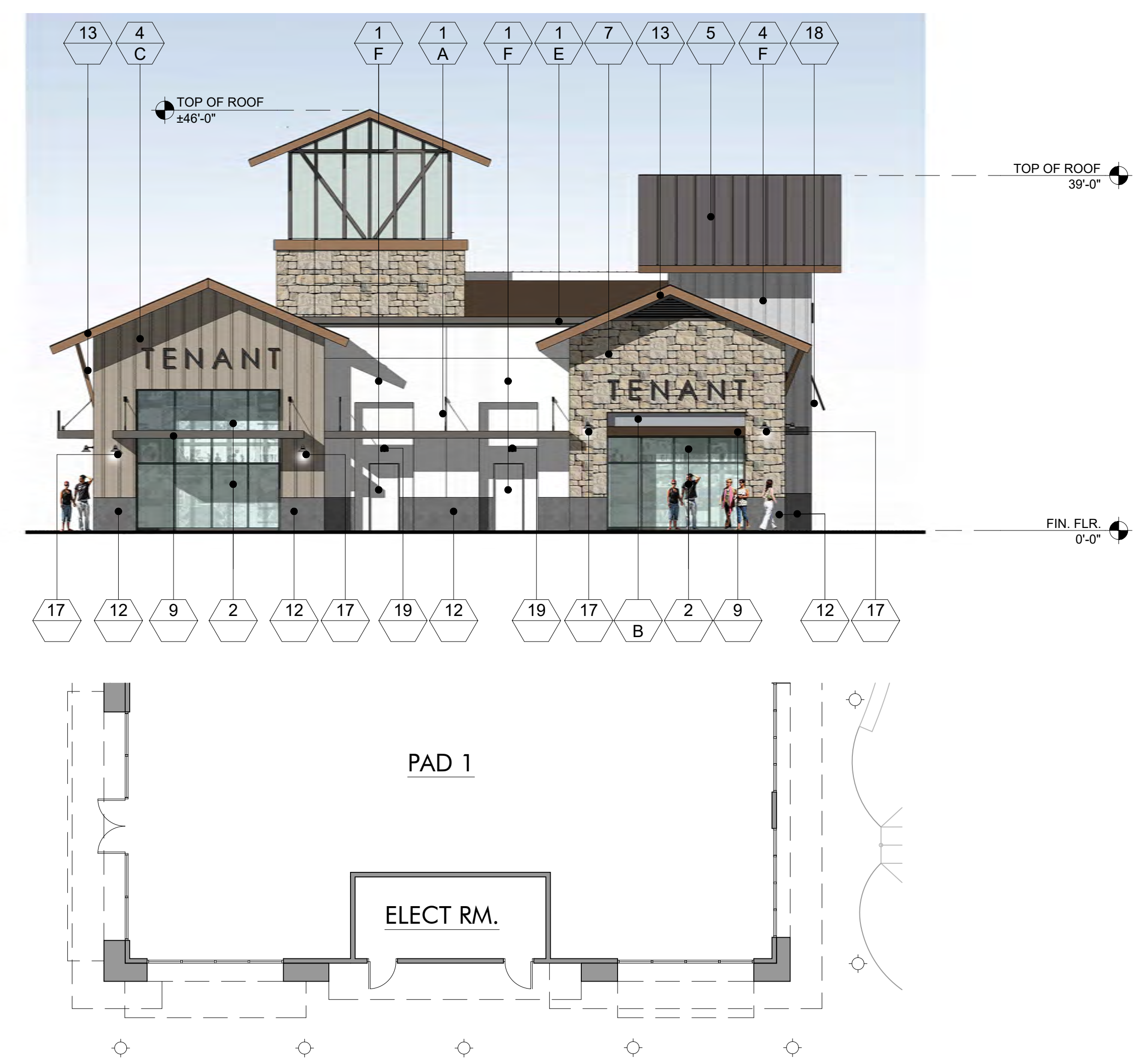
4 WEST ELEVATION - PAD 1 SCALE: 3/32" = 1'-0"
