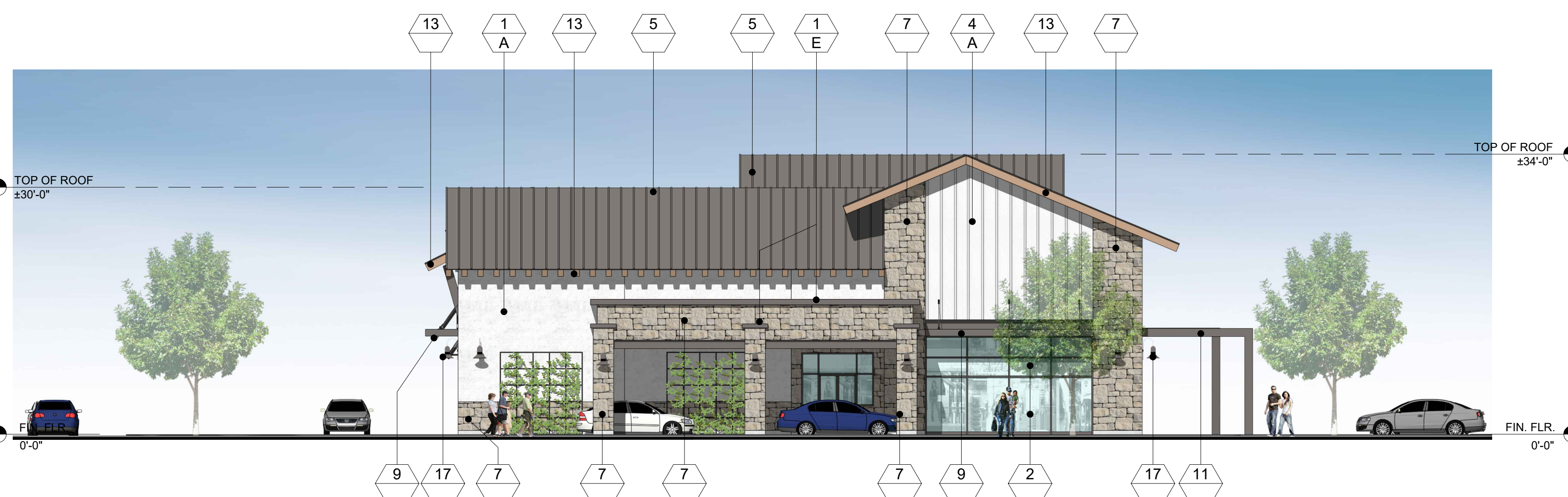
1 WEST ELEVATION - PAD 7 SCALE: 3/32" = 1'-0"
