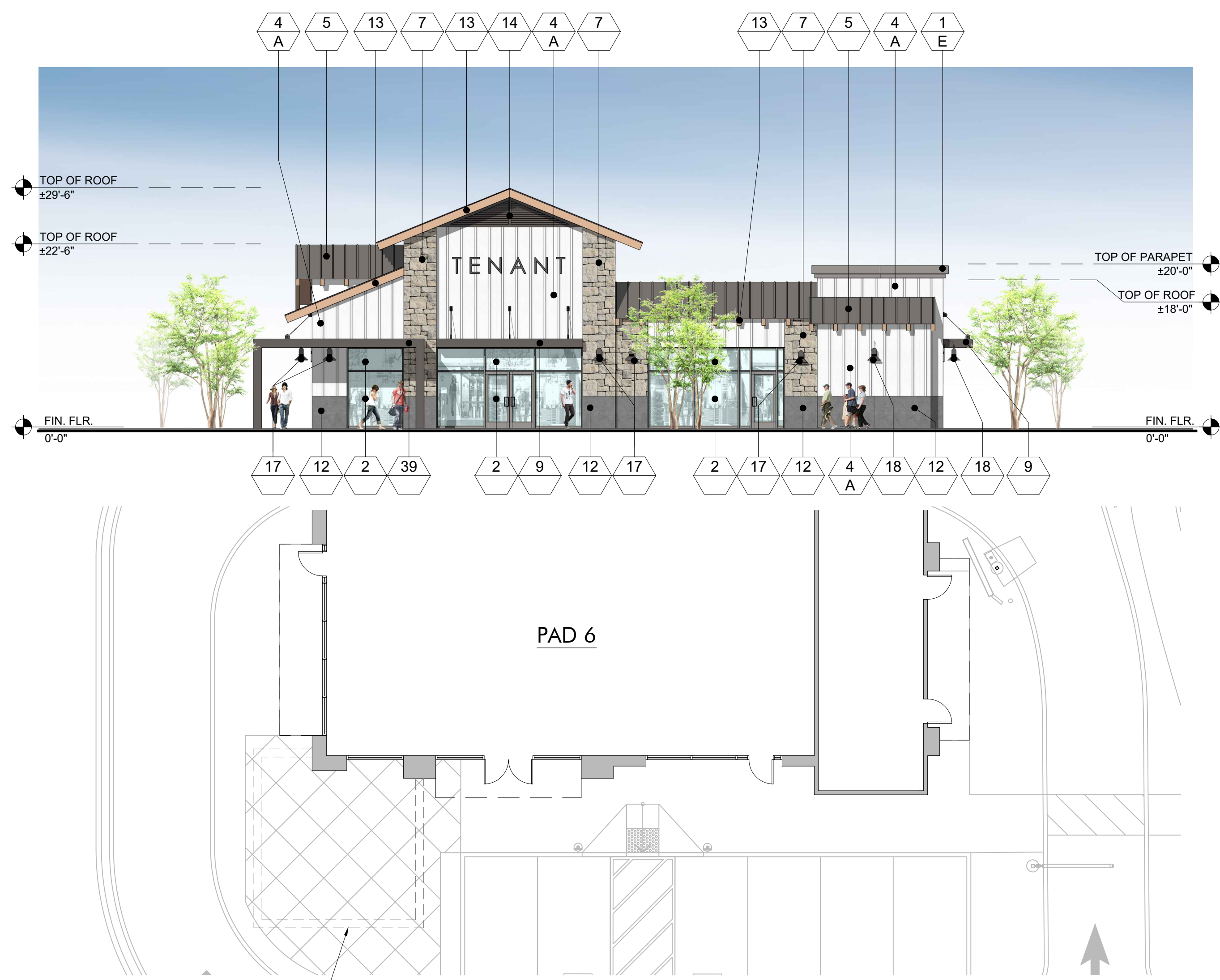
2 NORTH ELEVATION - PAD 6 SCALE: 3/32" = 1'-0"
