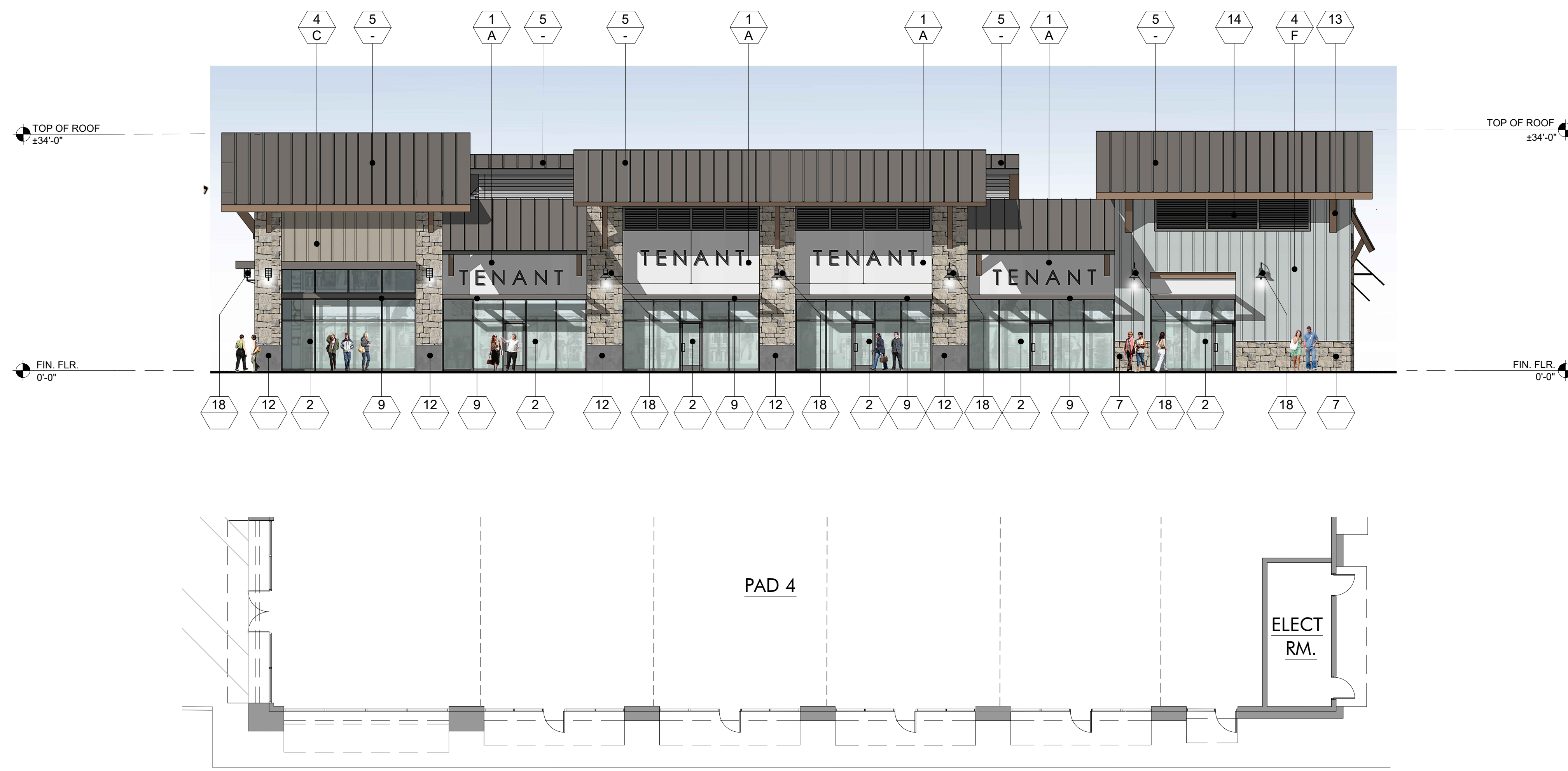
1 NORTH ELEVATION - PAD 4 SCALE: 3/32" = 1'-0"
