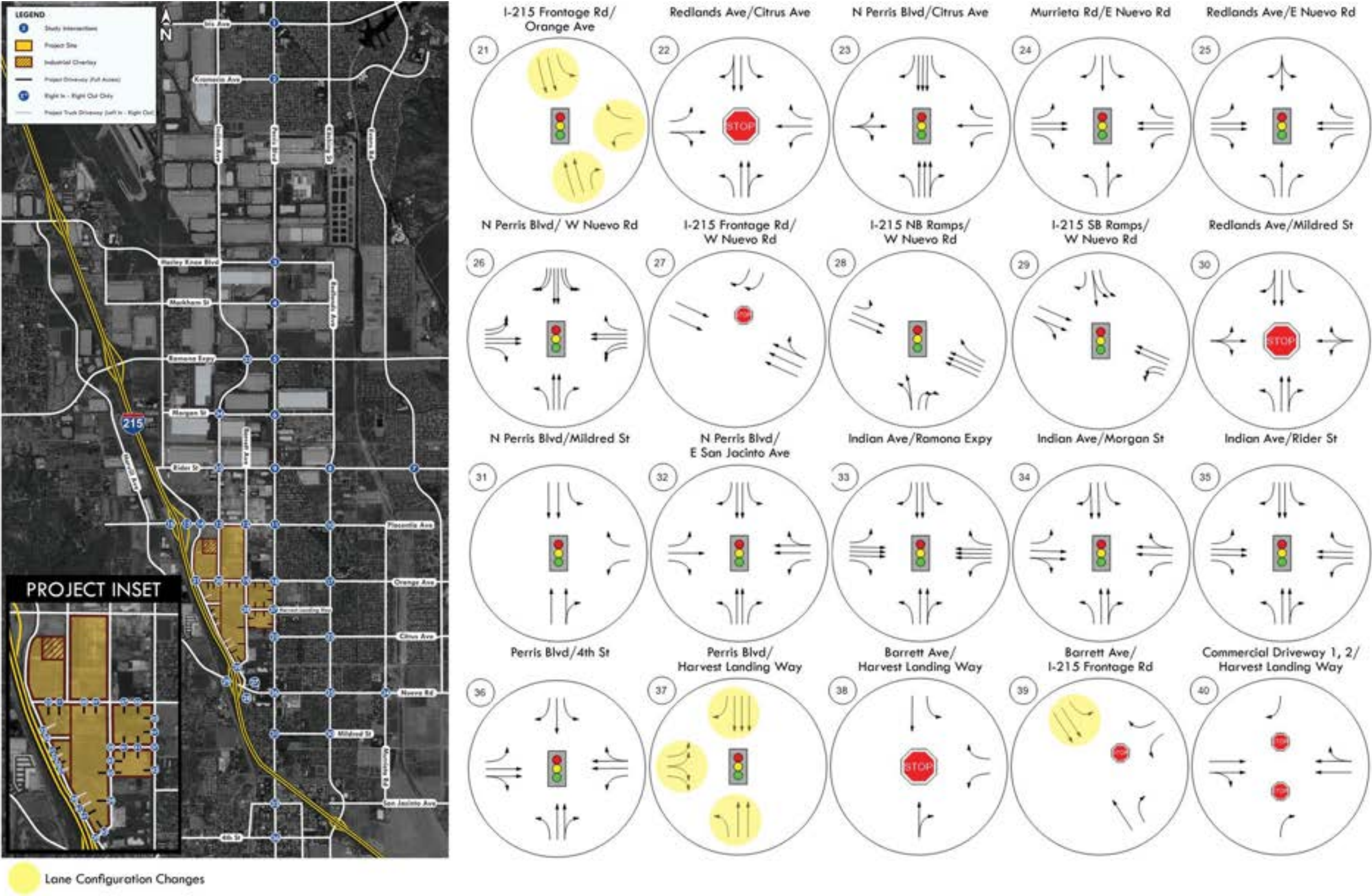
Figure 4.8b: Post-Project Completion Intersection Lane Configuration and Traffic Control (Continued)
