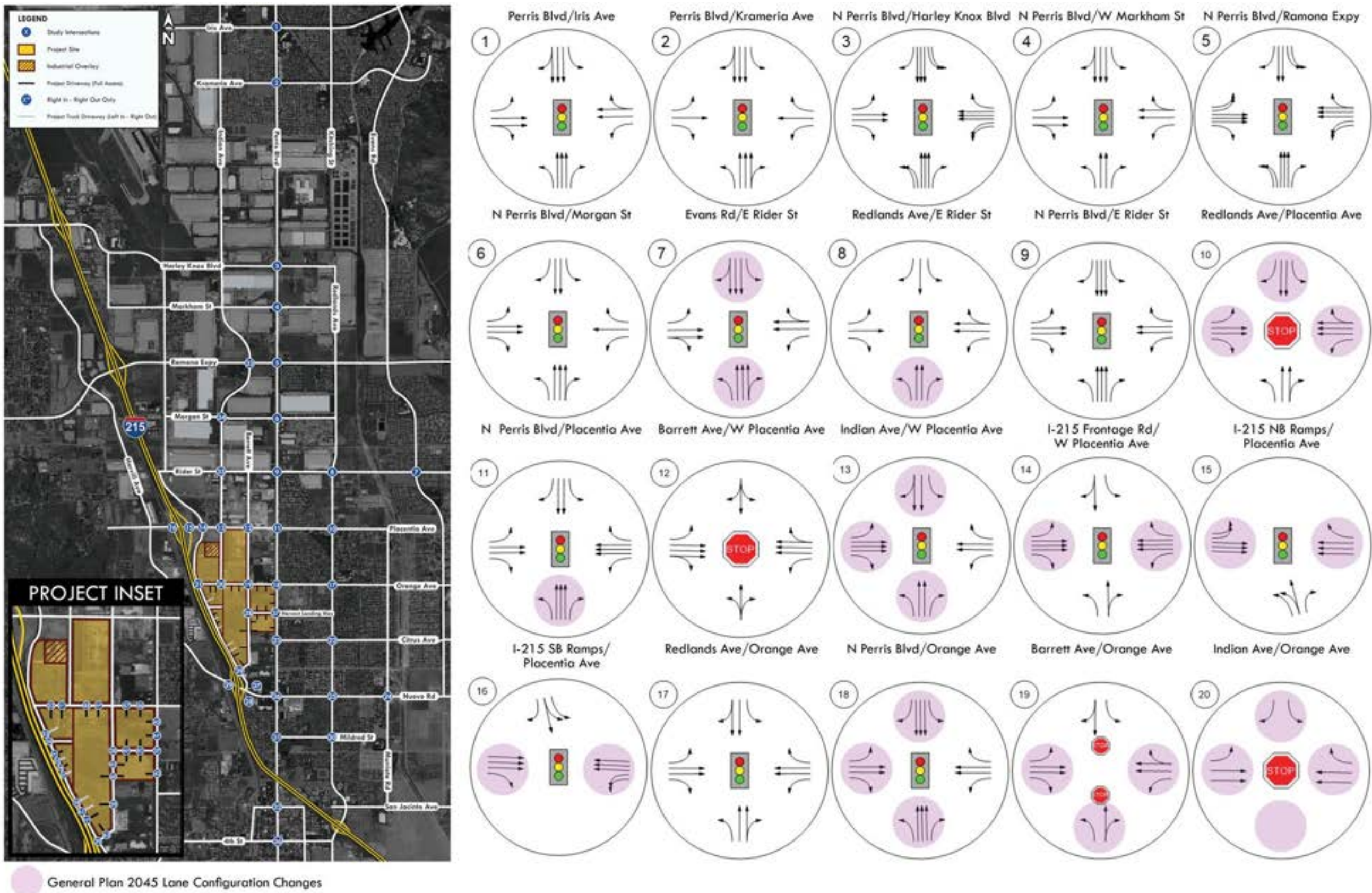
Figure 5.9a: General Plan 2045 Intersection Lane Configuration and Traffic Control
