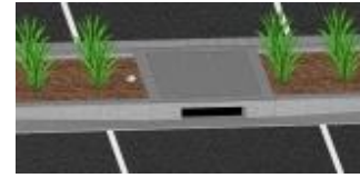
Horizontal Flow Biofiltration System
