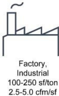
Figure 1 Industrial Building Cooling Load, Rule of Thumb 7
