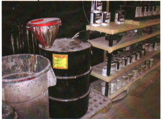
Flammable waste paint related material drum
