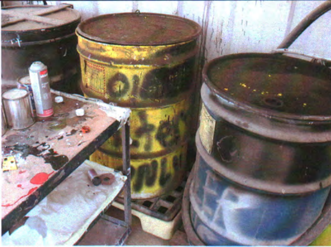
Used oil drum with hazardous label not filled out
