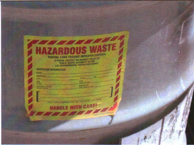
Hazardous waste label not filled out
