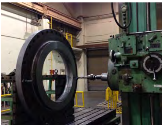
42" x 30" adapter flange being drilled at Metropolitan's La Verne Shops
