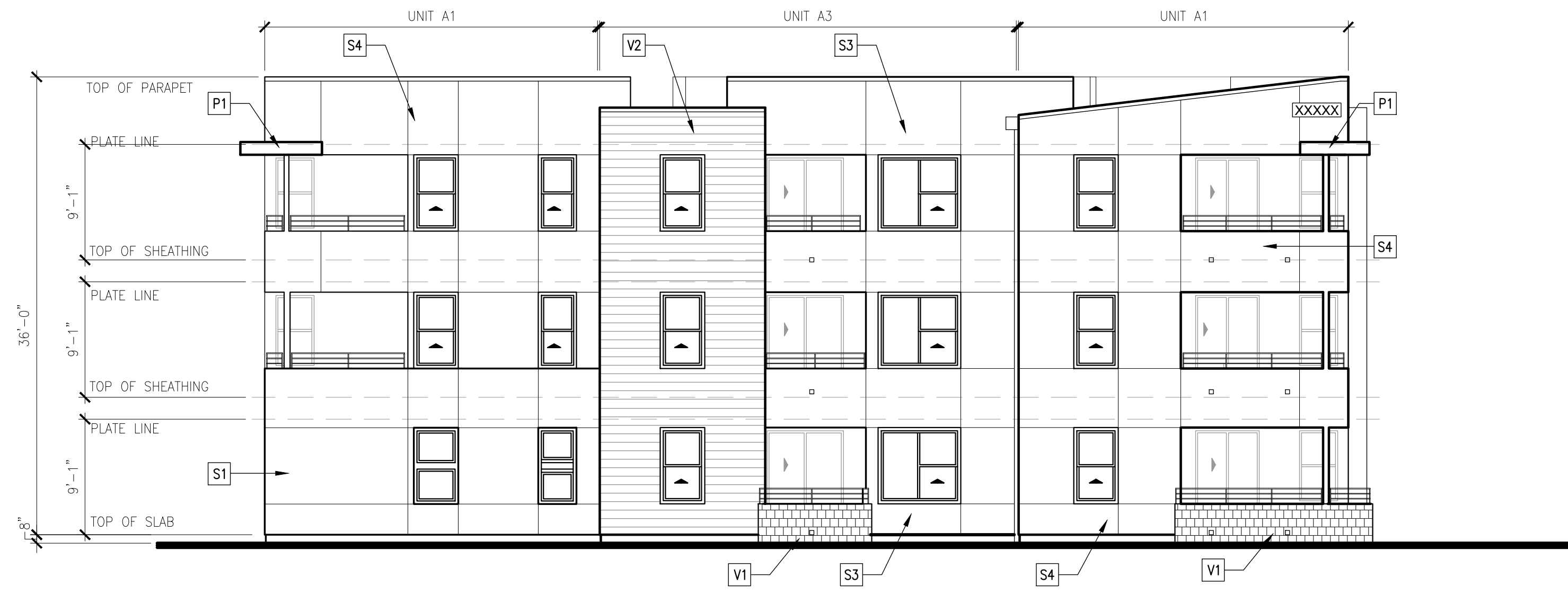
3 BUILDING TYPE 1 - SIDE ELEVATION
