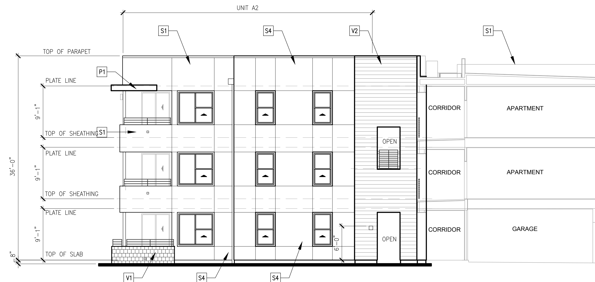
6 BUILDING TYPE 2 - COURTYARD ELEVATION AND SECTION
