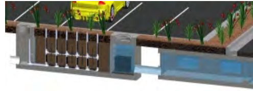
Horizontal Flow Biofiltration System
