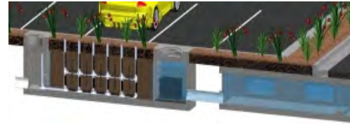
Horizontal Flow Biofiltration System
