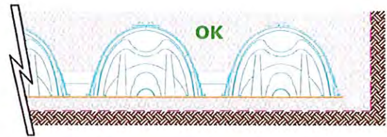
PERIMETER FULLY BACKFILLED CORRECT INSTALLATION
